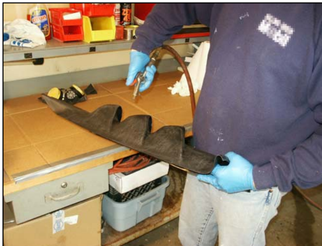
Figure 5) Blow off with compressed air
